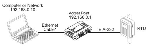
\*Use crossover cable for computer; straiht-through cable for network
